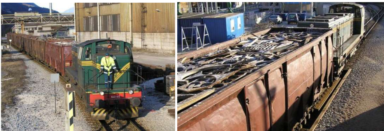
Figure 10: Shunting operations with 4-axle diesel locomotive and “Eas” freight wagons at iron factory Source: Acroni Jesenice
