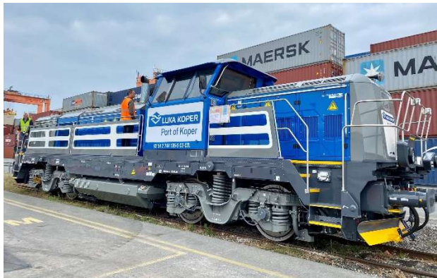
Figure 12: New shunting 3 and 4 axle diesel locomotives at Port of Koper Source: Port of Koper
