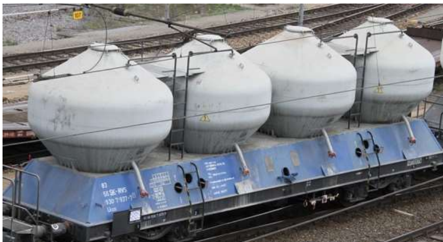
Figure 20: Railway wagon type Uacs Source: UNIZA
