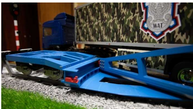
Figure 24: Innovative railway wagon with a low rotatable loading platform
