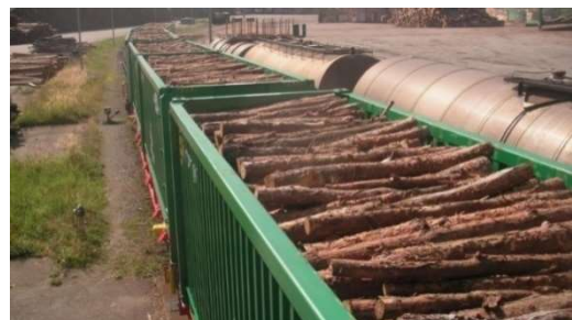
Figure 26: InnoWaggon 80 feet + WoodTainer XXL wagon with a payload capacity of up to 62 tonnes Source: RCH
