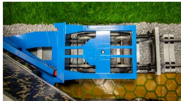
Figure 24: Innovative railway wagon with a low rotatable loading platform
