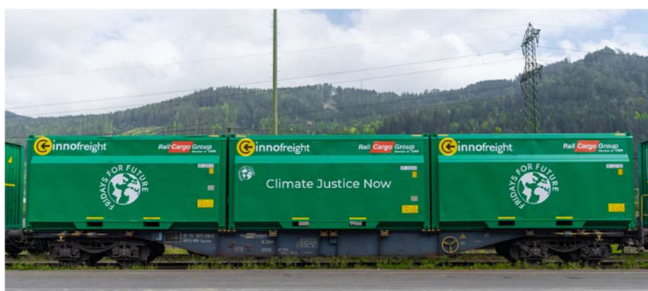
Figure 26: InnoWaggon 80 feet + WoodTainer XXL wagon with a payload capacity of up to 62 tonnes Source: RCH
