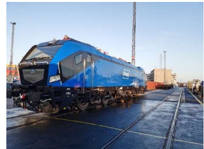
Figure 22: multi-system electric locomotive BISON Source: RCH
