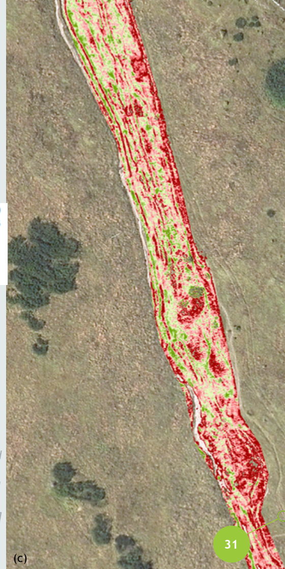
(a) TIN model from point cloud (b) and (c) show the change in the course of the hiking trail between the 2023 and 2024 seasons in the form of mass loss and mass gain, respectively [Authors]
