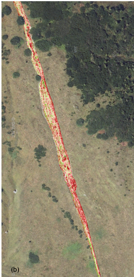
(a) TIN model from point cloud (b) and (c) show the change in the course of the hiking trail between the 2023 and 2024 seasons in the form of mass loss and mass gain, respectively [Authors]
