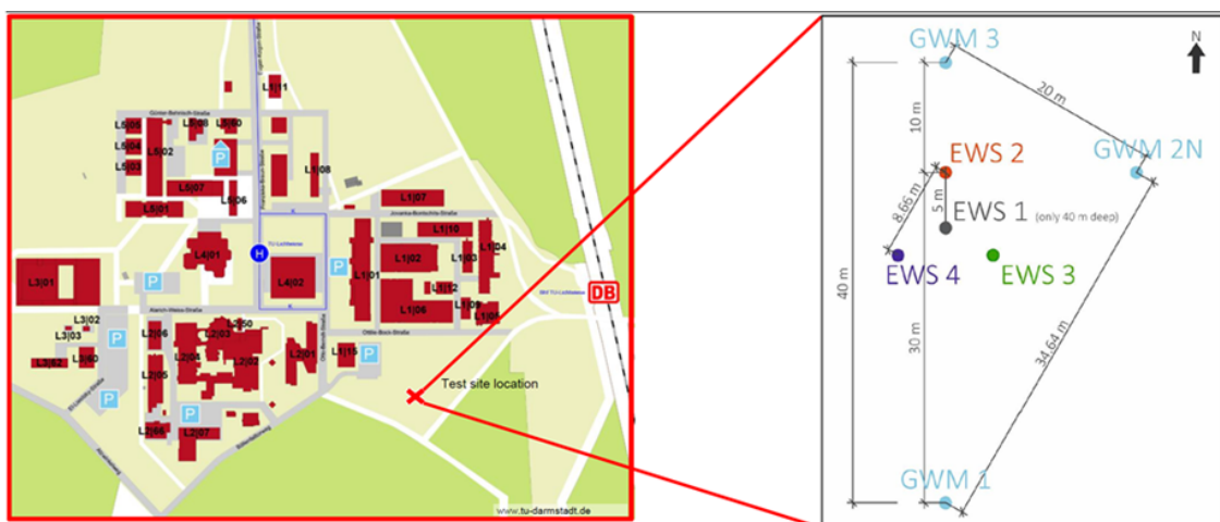
Figure D 12: Site location of the MD-BTES at the pilot site Campus Lichtwiese, TU Darmstadt ( www.push-it-thermalstorage.eu/pilots/darmstadt/ ).
